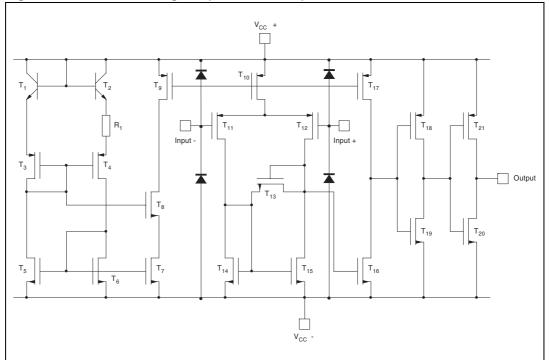
Figure 1. Schematic diagram (for 1/2 TS3702)
